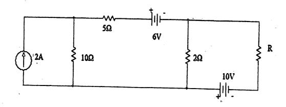
(c) Find the current through 5  $\Omega$  resistor using nodal analysis.
