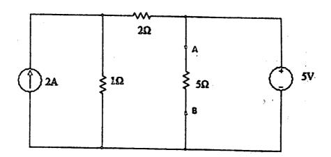
(b) Find R to have maximum power transfer in the given circuit. Also obtain the amount of maximum power transferred.
