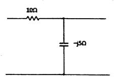
(a) Find the Thevenin equivalent of the given circuit. Determine the current through 5 Ω load resistor. Justify that the Thevenin equivalent circuit is equivalent to an ideal voltage source.
