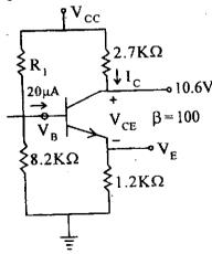
Determine  $V_{CE}$ ,  $I_C$ ,  $V_{CC}$  and  $R_1$ .
