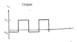
where  $V_{\rm D}$  is the voltage drop across forward biased zener diode,  $V_{\rm Z}$  is the reverse breakdown voltage of zener diode or zener voltage. Draw the circuit required to get the above output. (5)
