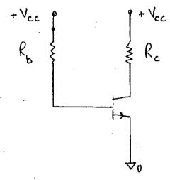
Given:  $R_b = 240 \text{ k}\Omega$ ,  $R_c = 2.2 \text{ k}\Omega$ ,  $V_{CC} = 12 \text{ V}$ ,  $V_{BE} = 0.7 \text{ V}$  and  $\beta = 100$
