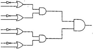
(c) Show how an AND-gate can be replaced by a suiable interconnection of OR-gates and NOT-gates.
