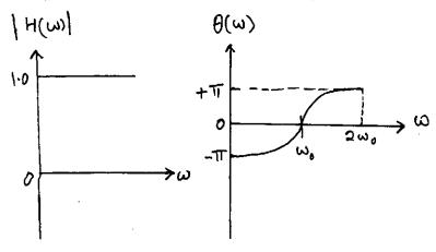
If the input signal applied to the network is  $v(t) = \sin \omega_0 t + \frac{1}{2} \sin 2\omega_0 t$ , write the expression for output voltage  $v_0(t)$  and plot it.
